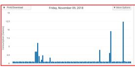
Water allows him to monitor his water usage online hourly, if he wishes, Entranosa members can upgrade to Eye On Water by paying a one-time fee to change out their meter and opening an account. Here is Steve's story: For three days, the Eye On Water program detected a flow of 1.2 – 2.0 gallons per hour (gph), which exceeds the maximum threshold of 1.0 qph. This graph shows what the leak looks like on the Eye on Water program. The continuous short bars are the leak (.6 gallons/15
