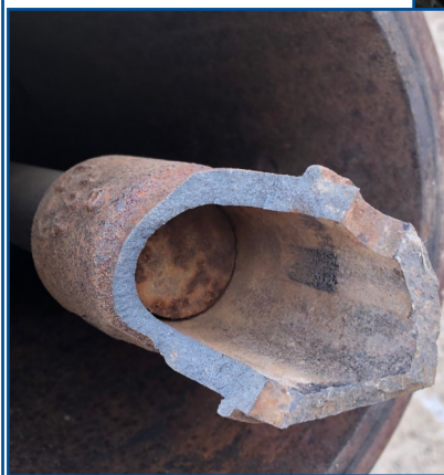
Hydrant Base Broke Away
