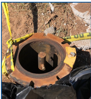
Hydrant Base Broke Away
