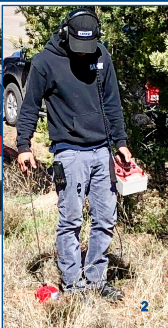
2 — Using specialized headphones, the technician listens for the sound of a leak
