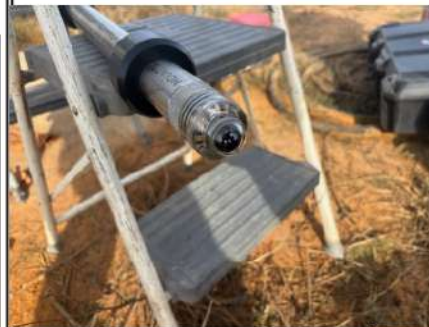
Wireless camera (above) records a high-quality video at depths up to 5,000 feet
