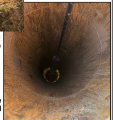
Wireless camera (above) records a high-quality video at depths up to 5,000 feet
